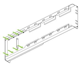
to adjust the length of the side-panel. 2 Adjust the rack side panel to fit the rack. Loosen eight (8) screws
